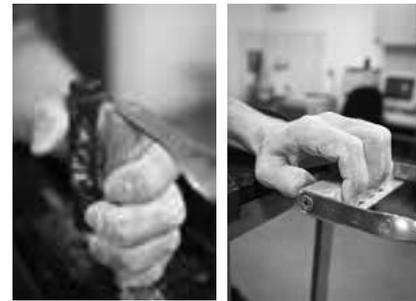
Figure 1. Position of the hand on the test stand during the measurement of maximum grip force ( $F_1$  – left,  $F_2$  – right)
