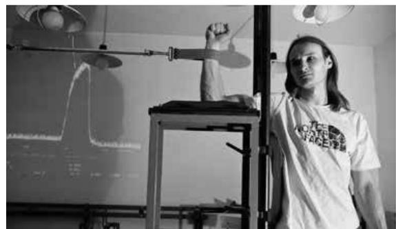
Figure 2. Maximum force development in the elbow flexors ( $F_{1_E}$ )
