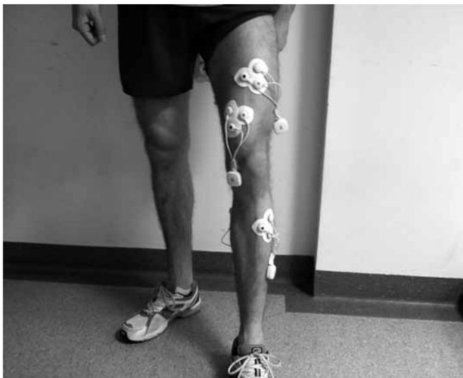
Figure 1. Lower limb with electrodes and wireless signal receivers
