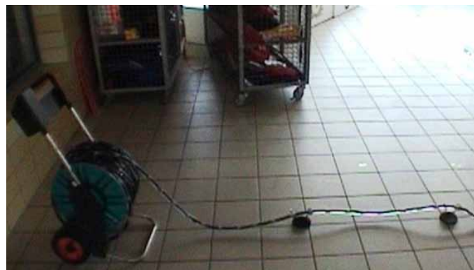
Figure 1. Leader device (Kuca Ltd., PL): a) controller, b) arterial tube with LEDs
