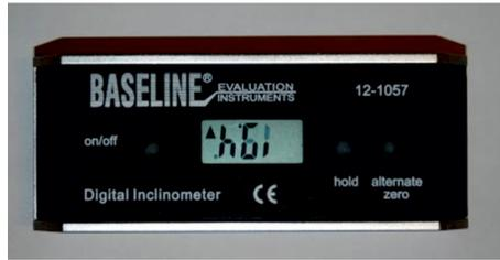
Figure 1. Saunders digital inclinometer (own photograph)
