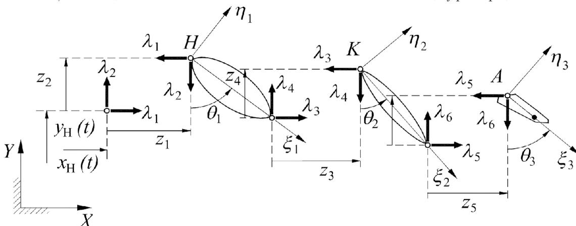
Figure 3. The kinematical chain of the right lower limb, the open-constraint coordinates, and the respective reaction forces
