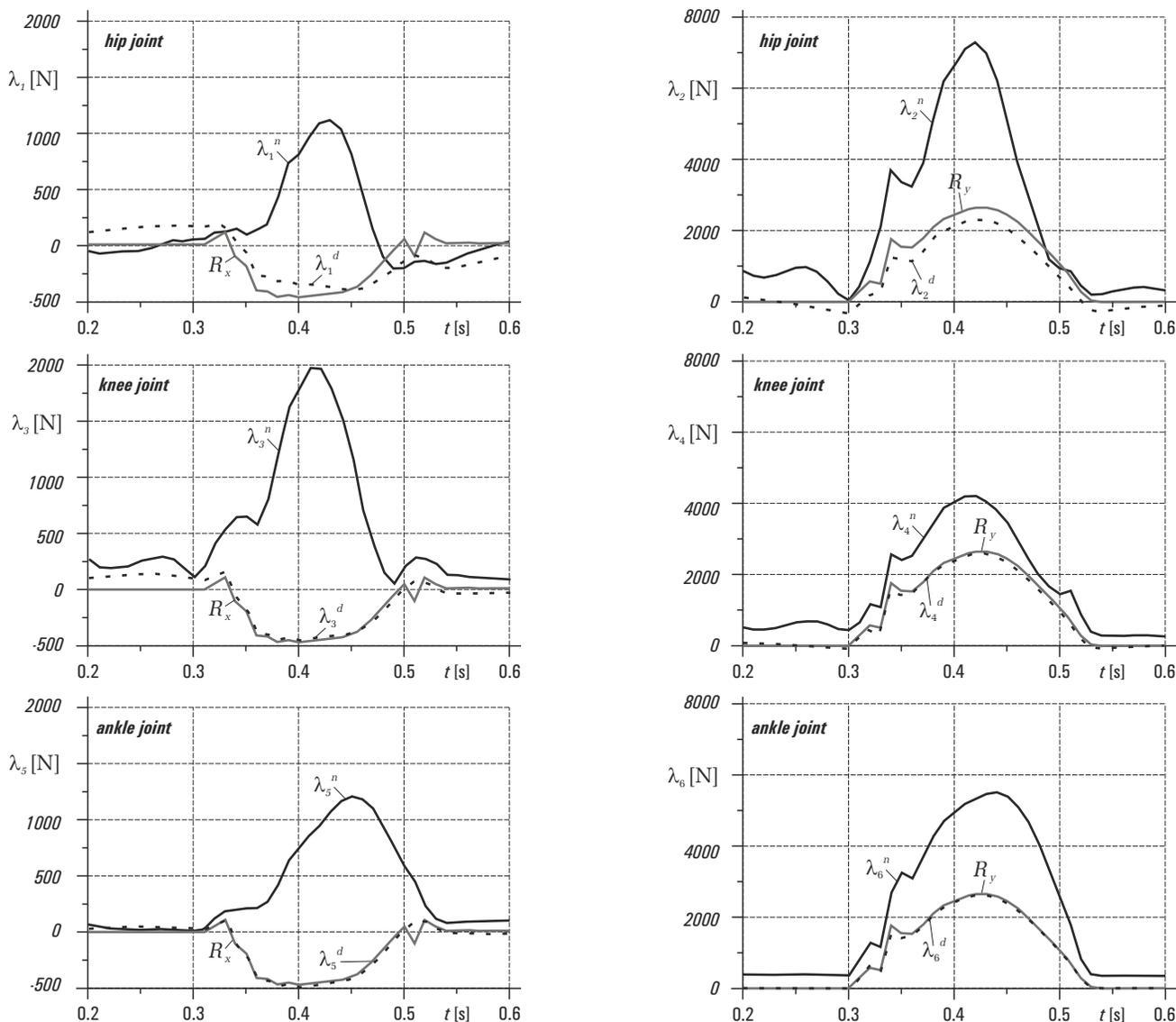
**Figure 5.** Reaction forces in the model joints obtained using the deterministic and nondeterministic models of actuation, versus the measured ground reactions (in grey): left column – the horizontal reaction components, and right column – the vertical reaction components (please notify the different scales in the graphs for the horizontal and vertical reaction components)
