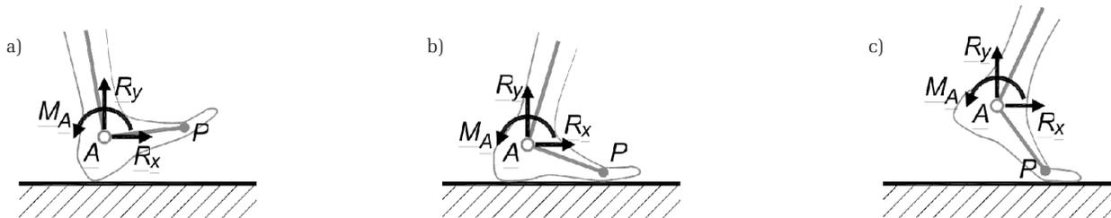
Figure 4. Possible scenarios of the foot contact with the ground, and the components of the external reactions on the foot reduced to the ankle joint A
